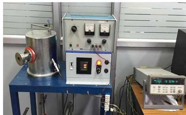
Fig. 1 Gas sensing measurement with DAQ system
